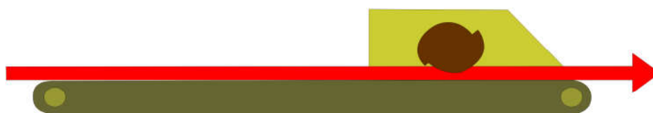
Impact roll crusher with horizontal material flow
